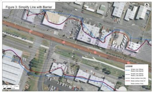
Figure 3 shows how this can be used. The Red line is the decibel (dB) 57 contour, it is included in the method as a barrier, to prevent the simplify line from the 56 dB contour line going across the 57 dB contour. The light Blue line has a tolerance of 50 metres and the dark blue line only has 10 metres tolerance. This should prove very useful when it comes to proving a planning line from noise contours.
